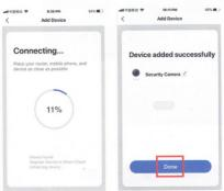
if device installation failure ,please use Other Mode: Smart configuration
